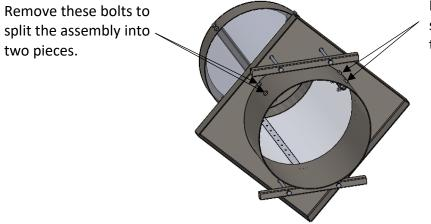
Remove these bolts to split the assembly into two pieces.
